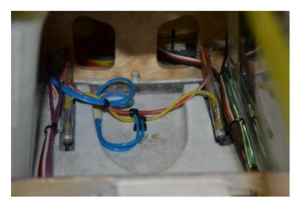
Assemble the fuel tanks, check for leaks and then check that they fit correctly into the forward section of the fuselage – it is quite tight to get the tanks into place but do persevere, it can be done. Once satisfied the tanks can be glued into place using a silicon sealant or similar, ideally only gluing around the exposed edges, so that a flexible long bladed knife can be used to cut the tanks free if they need to ever be removed at a later date.
