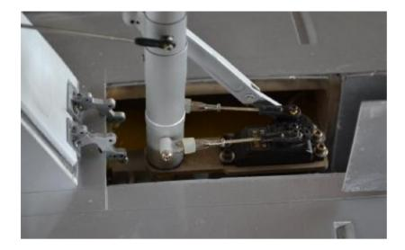
Refit the nose retract unit into the model – note that prior to fitting thin cyano glue can be poured into the screw holes in the retract unit mounting plates to toughen the wood. Make sure the glue is completely cured before finally re-fitting the nose retract unit.
