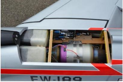
Fit the supplied air ducting as required, cutting it down to suitable length to allow for installation. Continue the installation of the remaining on-board equipment, the prototype used a Robbe PSS2018 twin receiver/battery system being powered by 6.6v 3000mAh Li-Fe batteries. Note the use of a MAP header tank to ensure a consistent and bubble free supply of fuel to the turbine.
