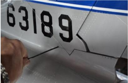
The extension leads for the rudder and tailplane servos should be retained to the fuselage sides so that they are well away from the tailpipe, using commercial servo lead mounts or by wrapping the leads in paper masking tape and then using cyano to glue the masking tape to the fuselage. It is suggested that the extension leads used are the correct length to enable all the connections to be made at the fuselage joint, as this makes assembly/disassembly of the fuselage much simpler.
