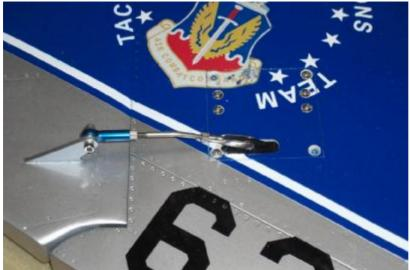
The rudder servo lead runs out through the bottom of the fin and into the fuselage, where it connects to an extension lead. Fit the fin/rudder assembly to the fuselage and securely tighten the fin post clamping screws.
