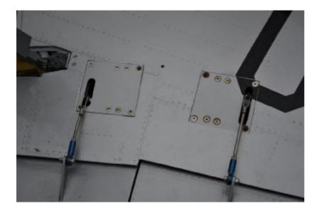
The slat servos should now be fitted to their hatch mounts, after which the pushrods should be made up and then connected to the horns pre-installed within the slats. Adjust the lengths of the pushrods until the slats close and open fully, without the servos being stalled at either end of their travel - this is a little fiddly to complete so a reasonable degree of patience is required, do not try to do this job in a hurry!
